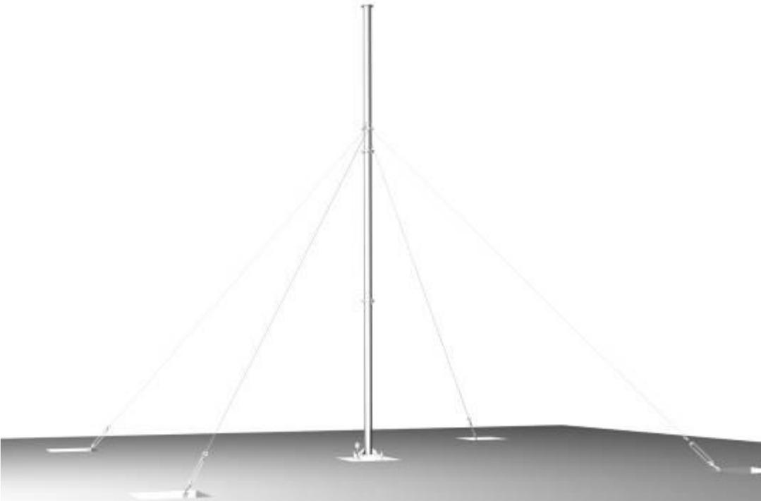
**3).** Reeve the wire thimble from top to raised face, make a circle around pole and through out (see fig), adjust the length of wire and tight with clip. Loose wire grip, pull up the pole; adjust the wire grid to keep the pole vertical.
