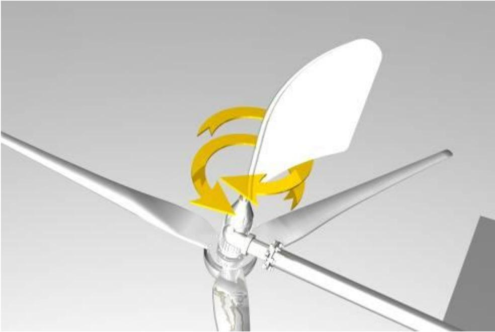
**B)** Fix the tail with four screws on back of generator.
