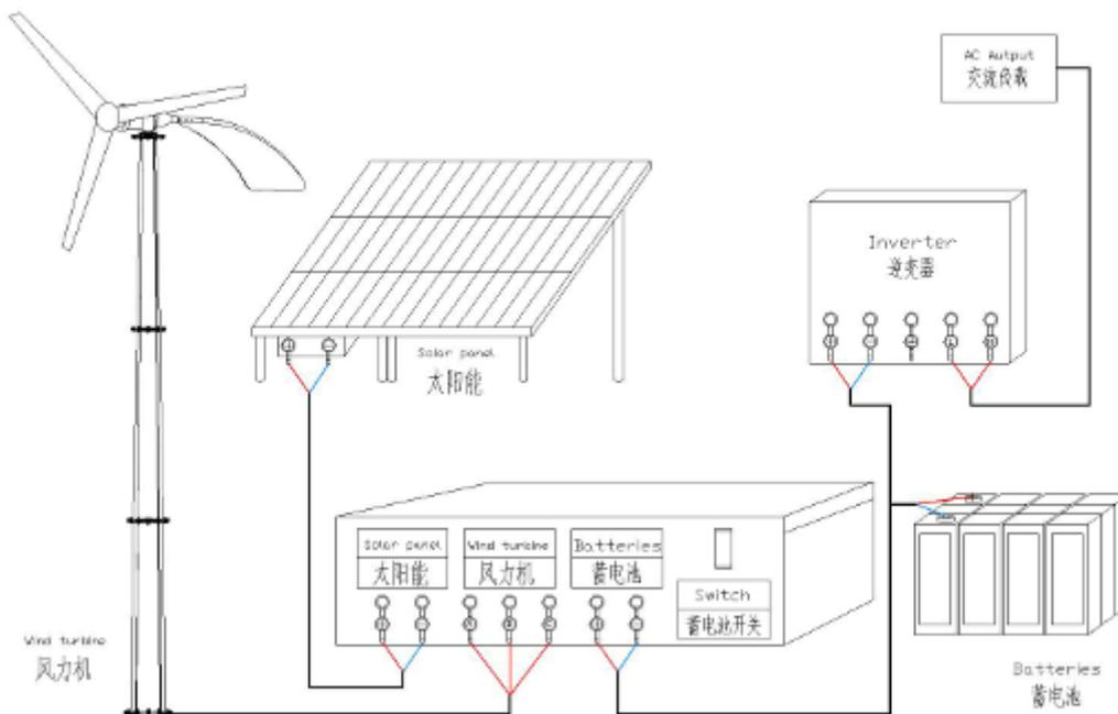
**D)** The red terminal of electrical box should be connected with “+” pole of battery. the black terminal should be connected with “—” pole of battery. Mustn’t be reversed. (Note: the voltage of battery should agree with the voltage of inverter and generator; the terminal should be connected firmly; to prevent corrosion, the terminal can be coated with oil or Vaseline)
