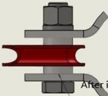
After installation the end face of hold hoop and sheath must unify closely, in case of bolt looseness
