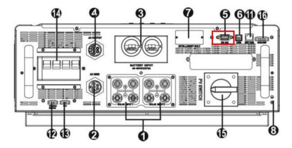
3. Please only connect AC GRID to inverter, make sure LCD is on after you turn on AC GRID switch. If utility icon is flashing, please exchange L2 and L3 input and check it again. If fine, please press "Enter" button for 1 sec at least to make it work in bypass mode as below.
